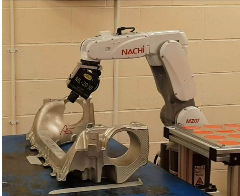
**Above:** Completely automatic inspection in strong daylight at 30 fps.
